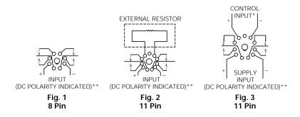
\* If control input is applied when supply input is applied, relay will immediately energize. A 50 millisecond minimum control pulse is required. \*\* Note Input polarity for DC operation. For most reliable operation on AC, connect high side to "+" and low side to "-".
